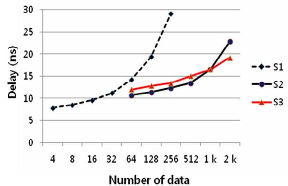
**Fig. 5.** Simulation results for the speed of SDWTA.
